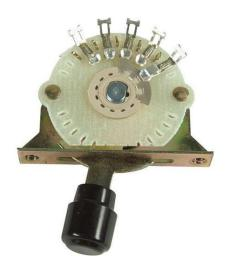
A pickup selector is a simple electronic switch that is hardwired to both the guitar pickups and eventually the guitar jack. When the switch is flipped in a direction, the switch connects the lugs wired to the pickups and the jack completing the circuit. This is how the pickups are selected. While one or a combination of pickups is selected, the other pickups are deselected by the same means.
