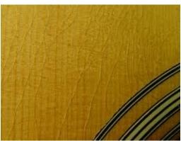
cause of cracks in the lacquer. When the temperature is changing, the wood will want to expand and contract. The lacquer will want to stay stiff, so when the wood is changing shape, the lacquer will crack. Lacquer cracks from the inside, so they will feel smooth if you run your finger across them if they haven't cracked all the way through.
