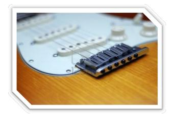
24.75". You can check the intonation by playing a fretted note on the 12th fret and then a harmonic on the 12th fret. These notes should sound exactly the same. If the note sounds sharp or flat, the intonation will need to be adjusted. At the bottom of each saddle is a screw that adjusts the saddle closer or farther away
