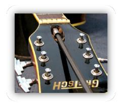
rod. The location varies on different guitars but is usually located at the end of the neck or behind a plate on the head. If your neck is bowed forward, you will want to tighten the nut to bend the neck backwards. If your neck is back-bowed, you will want to loosen the nut which will allow the neck to straighten or bow forward. As a rule of thumb, never adjust the truss rod more than 1/8<sup>th</sup> turn at a time. Over
