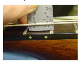
above the fret board are known as "High-action" the opposite goes for strings that are set low. The Action of a guitar is important when determining its playability. If the action is too low, then it can cause string buzzing. If the action is too high then it will start to become uncomfortable and difficult to play. So it's good to find a median where it is high enough to not cause
