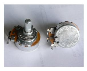
One of the parts commonly mentioned on electric guitars are the pots, but what exactly is a pot? Pot is actually short for potentiometer, a small device that controls the flow of electric current making it basically a glorified resistor. A guitar will usually have 2 pots; one is for volume and the other for tone. On the bottom of each pot
