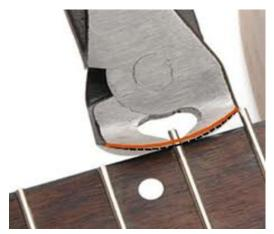
Nip the Fret Ends-After the glue has dried, you can take a pair of end nippers and cut off the edged of the frets that are hanging off the sides. After they are nipped off, you should take a file and smooth down the edges. Make sure to file downwards on the side of the board. If you file upward then you risk loosening your frets.
