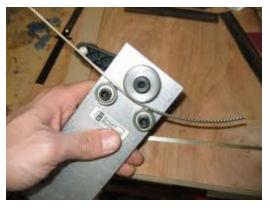
Fret wire will usually come in 1 or 2 foot sections, although they can be bought pre-cut. This fret wire will initially be straight but to fit it on to your guitar, your will have to bend it to the radius of your fret board. You can use a fret wire bender to correctly bend it to fit your fret board
